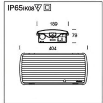
**Housing:** Vandal-resistant, self-extinguishing, UV-stabilized, anti-yellowing grey polycarbonate.
